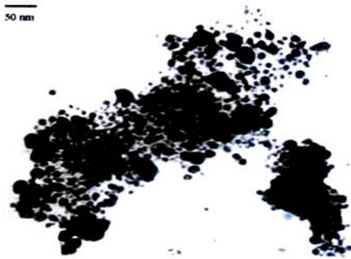
Fig 1.5: Transmission electron micrograph of silver nanoparticles
